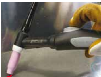
(4) Lay the outside edge of the Gas Cup on the work piece with the Tungsten Electrode 0.040" - 1/8" from the work piece
