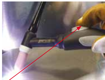
(5) Press the torch switch and the arc will ignite across the gap between the tungsten and work piece. Hold even distance of about 5/64" gap between the tungsten and work piece to maintain the arc.
